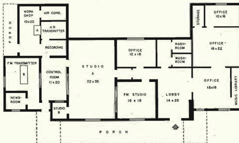
Floor layout for 250 watt a-m (A) and 3 kw f-m (B) transmitter at KGBS, Harlingen, Texas. W. O. Porter is chief engineer at this station.
